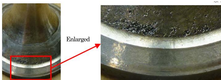
Photo 1. Intake Valve Corroded
